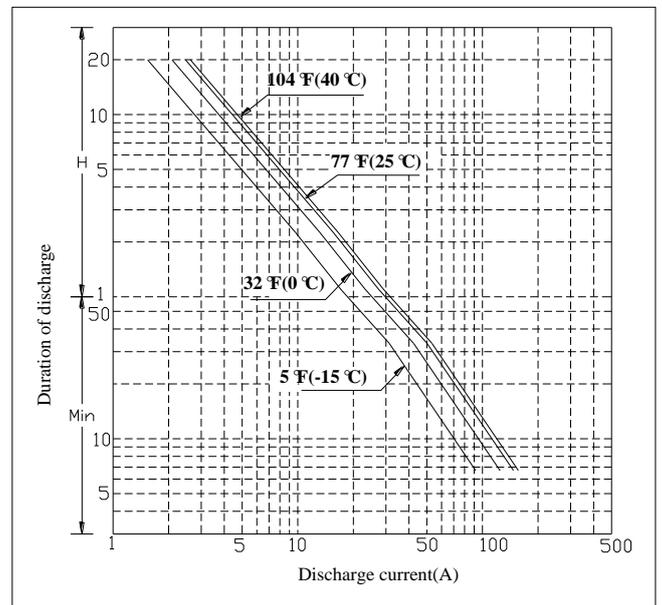
**Constant Current Discharge Rating Amperes @ 77 °F (25°C)**
