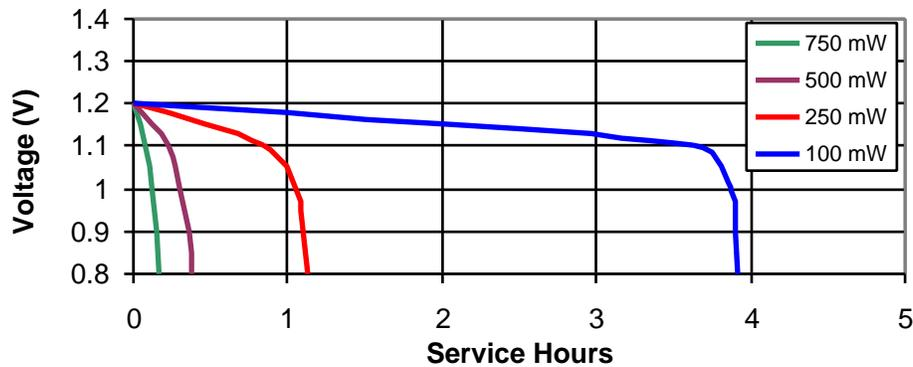
\* Delivered capacity is dependent on the applied load, operating temperature and cut-off voltage. Please refer to the charts and discharge data shown for examples of the energy / service life that the battery will provide for various load conditions.
